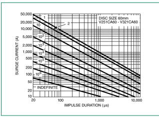
NOTE: If pulse ratings are exceeded, a shift of  $V_{\text{NIDC}}$  (at specified current) of more than  $\pm 10\%$  could result. This type of shift, which normally results in a decrease of  $v_{\text{NIDC}}$ , may result in the device not meeting the original published specifications, but does not prevent the device from continuing to function, and to provide ample protection.
